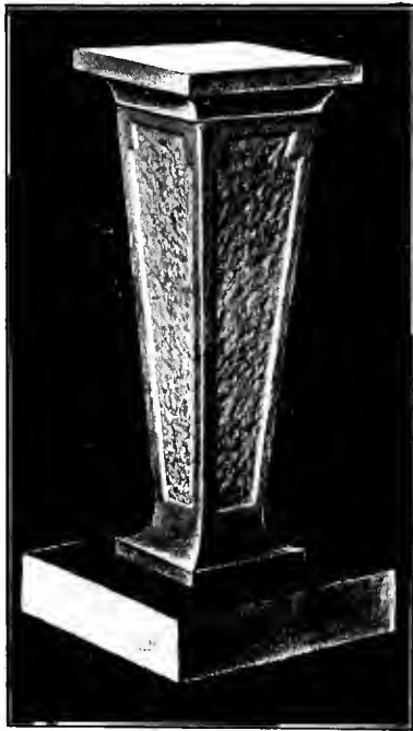
Fig. 93—Concrete Pedestal—Executed by the Author
